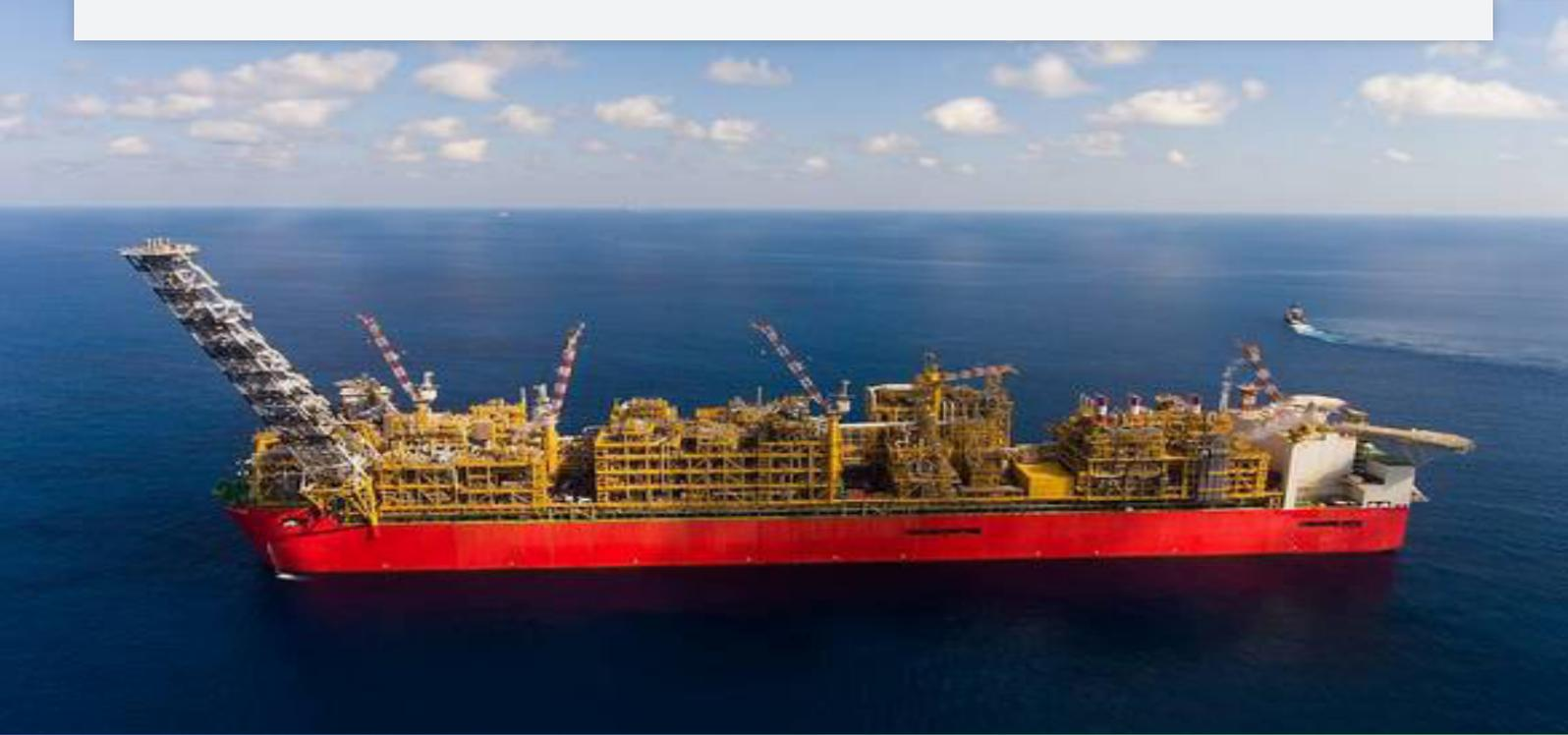
**Prelude FLNG is a liquid-rich gas field located in North-West Australia, 475 km North-North East of Broome, in approximately 240m water depth. The field subsea development includes 7 subsea wells, 4 production risers, and the world's largest umbilical. EnerMech secured the contract to provide services and equipment to undertake the pre-commissioning works on the risers, electro-hydraulic umbilical (EHU), electrical steel flying lead (ESFL), and electrical flying lead (EFL).**
